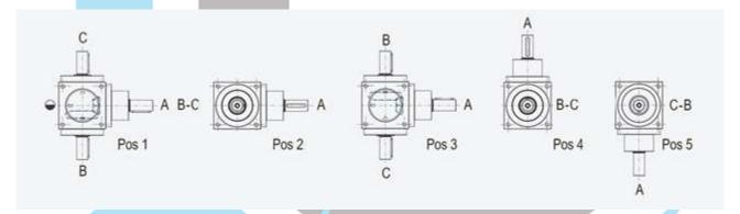
Pos. 2 and 5: does not require any particular attention, if not present any other special operating condition. In those cases, if oil level and type are correct, all the shafts, gears and bearings are correctly lubricated;
